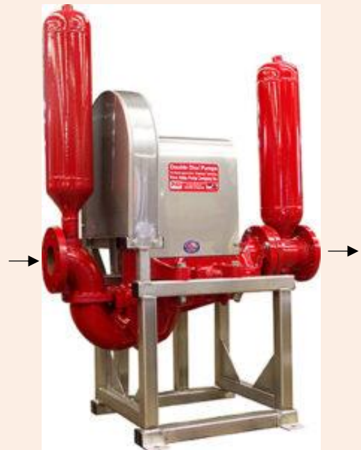
Figure 8: Left: Suction and discharge cycles of a double disc pump. During the suction cycle, the suction disc (on the left) rises and the clack valve opens to draw in fluid.
