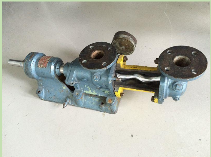
Figure 17: Left: Fluid flow shown in red as the rotor rotates inside the threaded stator. Right: Example of a small progressive cavity pump with the stator partially removed.
